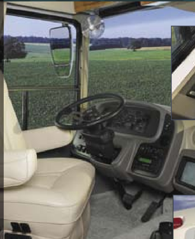
Push-button transmission shifter is featured on units built on W-24 chassis.
