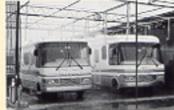
Each unit is thoroughly rain-tested before delivery. This important step helps assure a water-tight motorhome.
